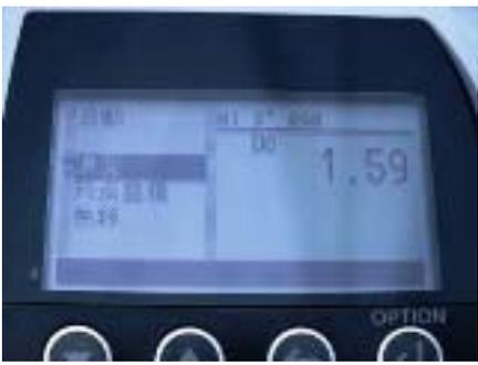
The image shows the screen after a solid color patch has been measured. The '測定' option is still highlighted. The screen displays '00' and a large number '1.59', representing the solid density.                                                                                         | <p>When a solid color patch is measured, the ink is automatically determined and the solid density is displayed.</p> |
