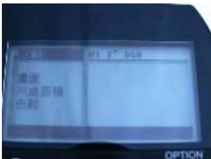
After 2 seconds, the screen will change to the measurement screen.
