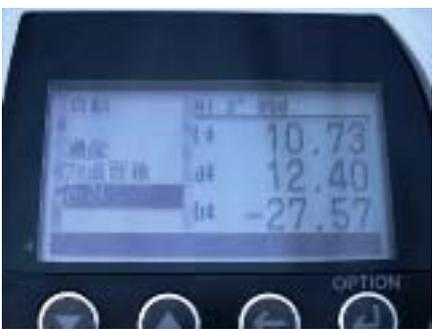
The image shows the screen after an over-print has been measured. The '測定' option is still highlighted. The screen displays '14', '10.73', '04', '12.40', and '14', '-27.57', representing the color values.                                                                            | <p>When the over-print is measured, the color is displayed.</p>                                                      |
