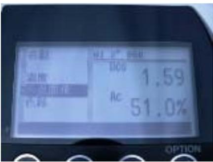
The image shows the screen after a solid color patch has been measured. The '測定' option is still highlighted. The screen displays '000', '1.59', and 'AC 51.0%', representing the solid density and the color (AC) and its percentage.                                                   | <p>When a solid color patch is measured, the ink is automatically determined and the solid density is displayed.</p> |
